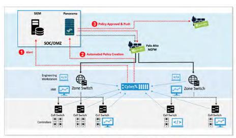
CyberX's integration with Panorama™ enables joint customers to rapidly block sources of malicious traffic in ICS/SCADA networks
